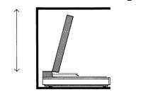
The record player must be placed horizontally on a stable surface. Allow a space of at least 30 cm above the record player so that the dust cover can open freely. Avoid placing it in direct sunlight or near radiators or other sources of heat.
