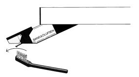
Carefully stroke the stylus from the back of the cartridge towards the front. Do not use any chemical fluids to clean the stylus.
